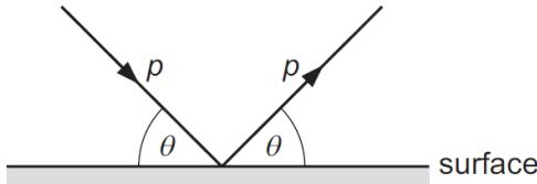
The ball rebounds with the same magnitude of momentum at an angle  $\theta$  to the surface. The ball is in contact with the surface for time  $t$ . What is the magnitude of the average resultant force acting on the ball during the collision?
