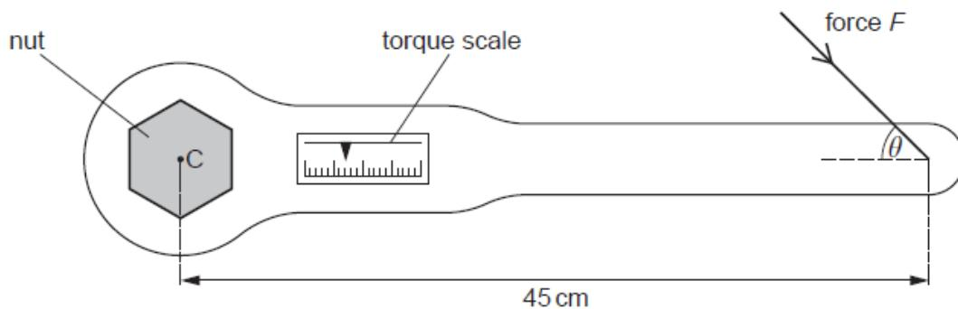
The wrench is put on the nut and a force is applied to the handle. A scale indicates the torque applied.
