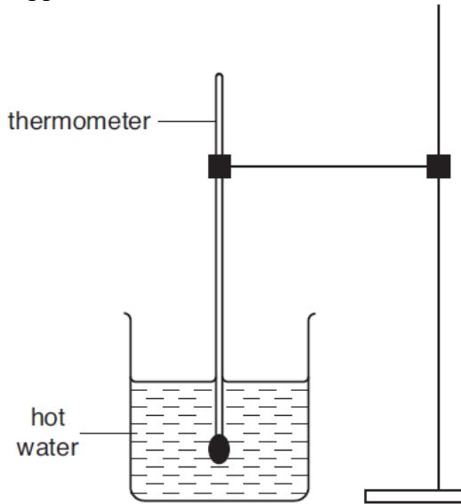
Hot water is poured into the beaker and temperature readings are taken as the water cools. Table 1. shows the readings taken by one student.
