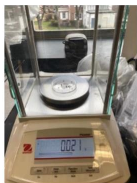
Figure 2: Analytical balance used to find the average weight of each of the fly types.
