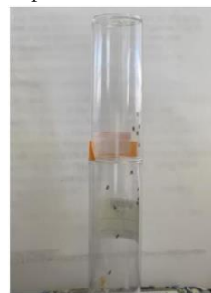
Figure 1: Negative Geotaxis Test tube made with 2 stacked culture vials.
