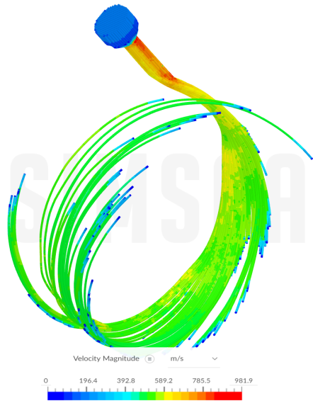
Figure 8 : The CFD simulation of all six vortex generators
