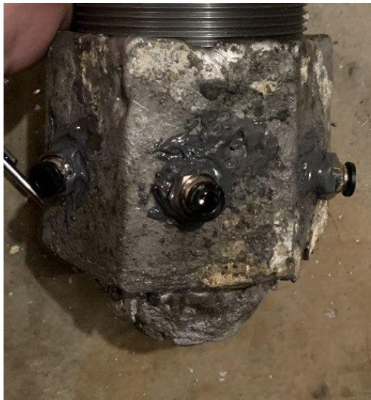
Figure 19: This is the nozzle I cast out of aluminum
