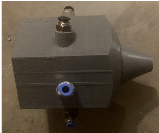
Figure 18 : The 3d printed nozzle
